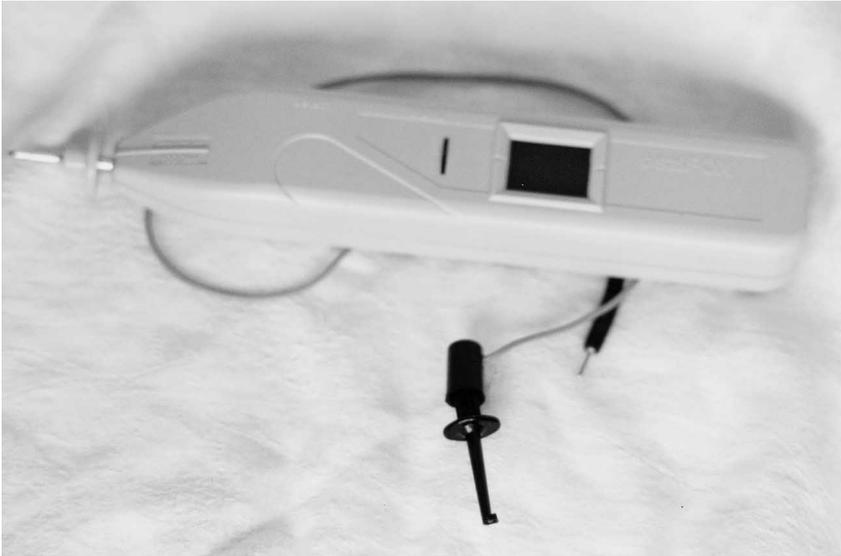
**Figure 215** OsziFOX hand-held digital oscilloscope
