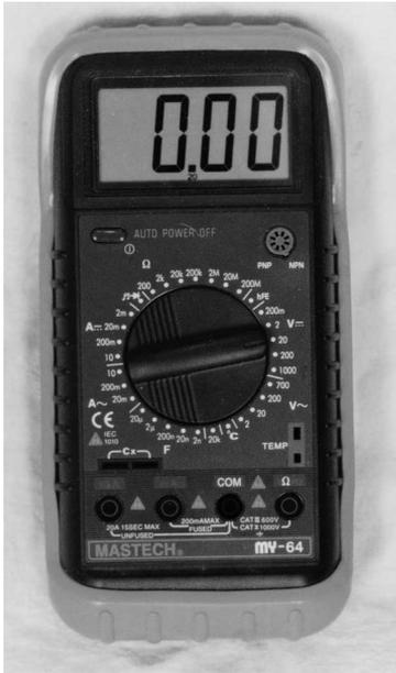
**Figure 205** Digital Multi-Meter (DMM)
