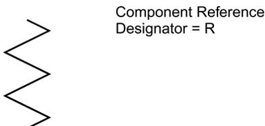
**Figure 22** Resistor symbol
