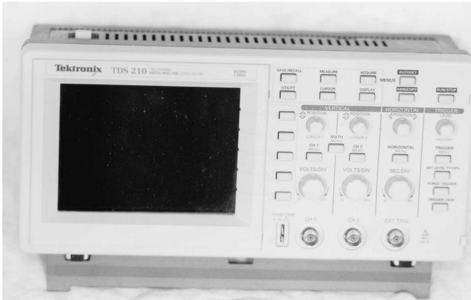
**Figure 211** TDS-210 digital oscilloscope
